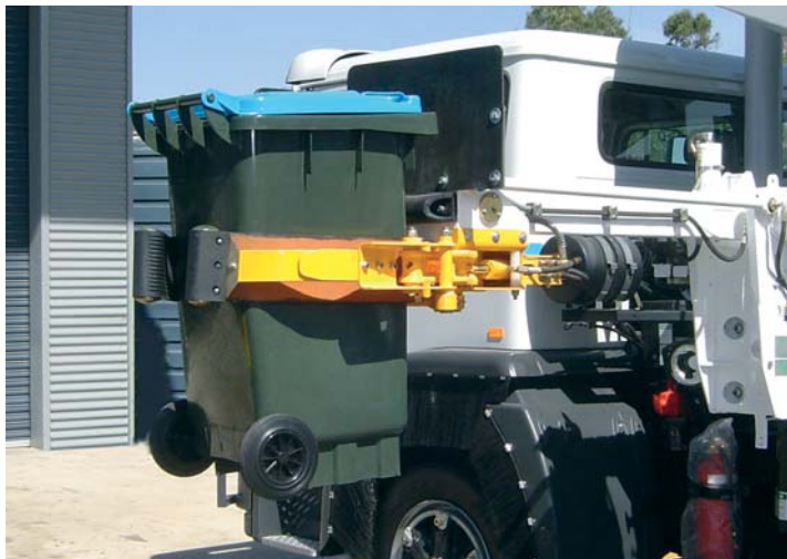
Above: One of the MASTEC® bins undergoing a PED:TC0010 Bin Lift Cycle Test at MJE's Adelaide facility.
