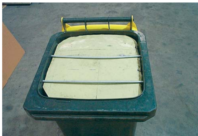
Above: The PED:TC0010 Bin Lift Cycle Test was first conducted on the MASTEC® 240-Litre MGB, which was loaded to a weight of 75kgs and then subjected to an equivalent of over 10 years of simulated lift activity with a 'grab-arm' side lift collection system.
